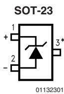
\*This pin must be left floating or connected to pin 2.
